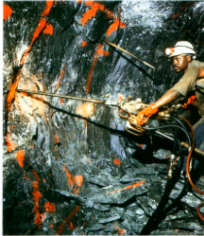
In hard-rock mining, which follows the path of gold vein through the earth, ore of payable grade is removed by hand-held pneumatic drill. When it is too dangerous for humans to perform the drilling, robots are increasingly being employed.
